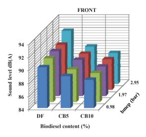
Fig. 4. Sound level at various loads for diesel fuel and biodiesel blends.
