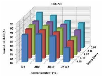
Fig. 4. Sound level for different fuel samples
