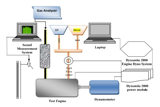
Fig. 1. Schematic diagram of test engine and setup
