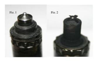
Fig 6. Carbon depositions in Injector tip after using a) No. 2 Diesel b) 95% No. 2 diesel & 5% palm olein.
