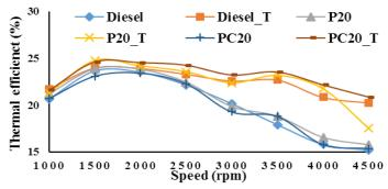
Fig. 5: Engine brake thermal efficiency at different speed
