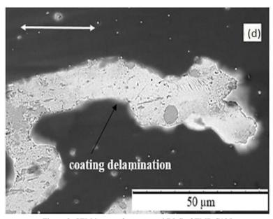
Figure 2. SEM image of un-textured DLC of TMP-C125
