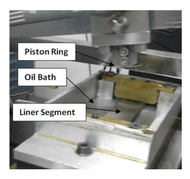
Fig. 8. Piston ring and liner specimen in reciprocating test rig
