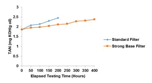
Fig.6. Total acid number of degraded oils after long hour tests.
