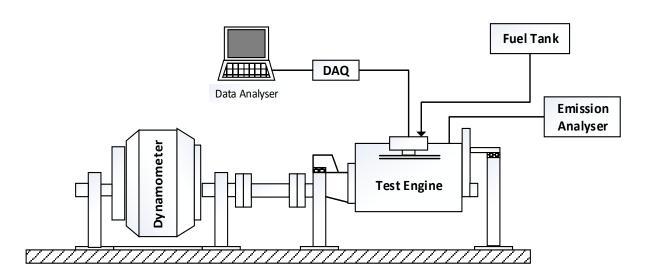
Fig. 4. Schematics of the engine test bench
