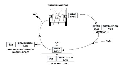
**Fig.7.** Mechanism for lubricant conditioning by strong base filter [24].
