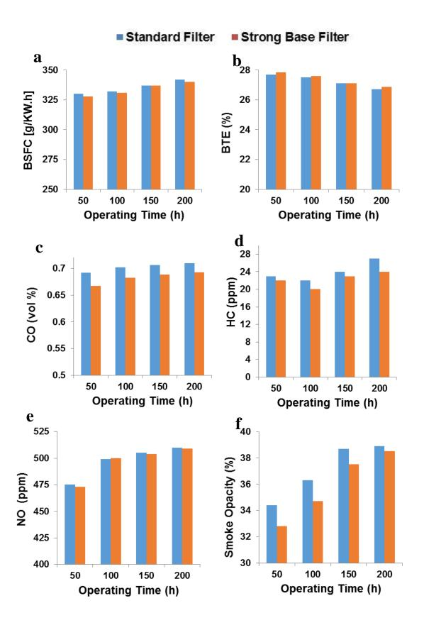
**Fig.10.** Fuel consumption and exhaust emissions during the long hour tests.
