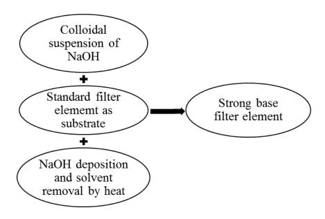
Fig.1. Schematic diagram for deposition of strong base on a standard filter element
