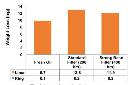
Fig. 9. Piston ring and cylinder wear
