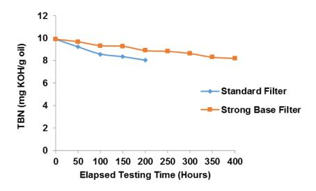
Fig.5. TBN retention of degraded oils after long hour tests
