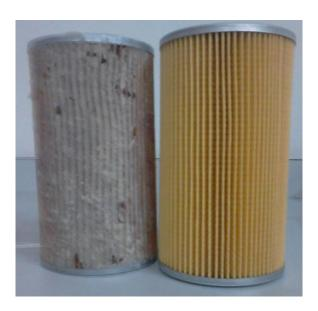
Fig. 2. Standard filter element and strong base (NaOH) filter element
