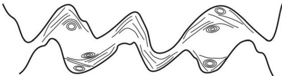
Fig. 16. Illustration of smoothing/polishing effect by filling up of rough valleys of rubbing surfaces (Kalin et al. 2012).
